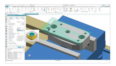
Machining simulation – to avoid tying up a machine in unproductive prove-outs, the integrated machine tool simulation provides a more complete simulation than most systems with its machine-code-driven motion. Smart Machine Simulation Kits are available via Post Hub for a wide variety of machine tools, and custom kits can be created.
