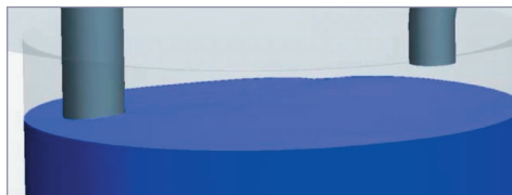
Figure 7. The air-water interface in the sump shows a low level of deformation, indicating no vortex formation or air entrainment.
