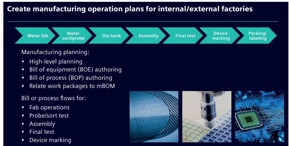
Figure 17. Industry-specific process flows for front-end and back-end manufacturing.
